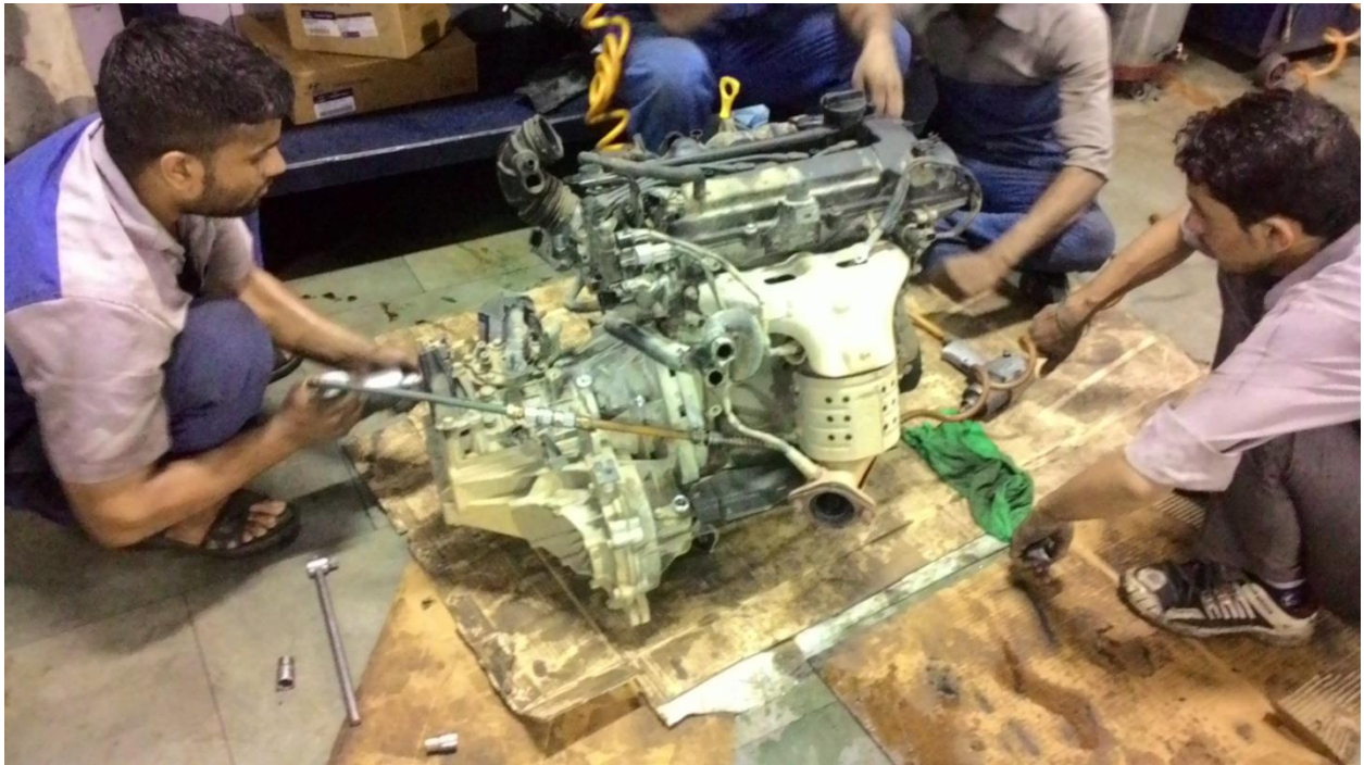
Fig. 3.8 Separating gear box from engine
