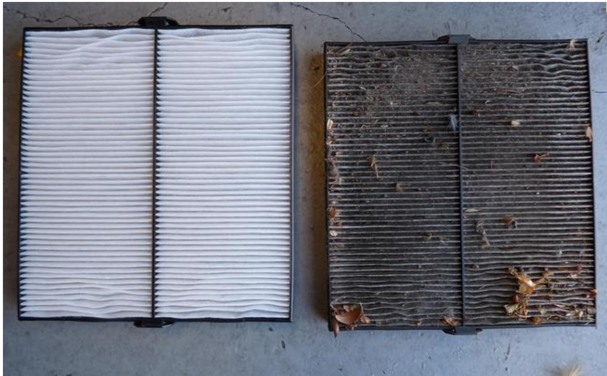
Fig. 4.2 Left side new a/c filter other side polluted a/c filter
