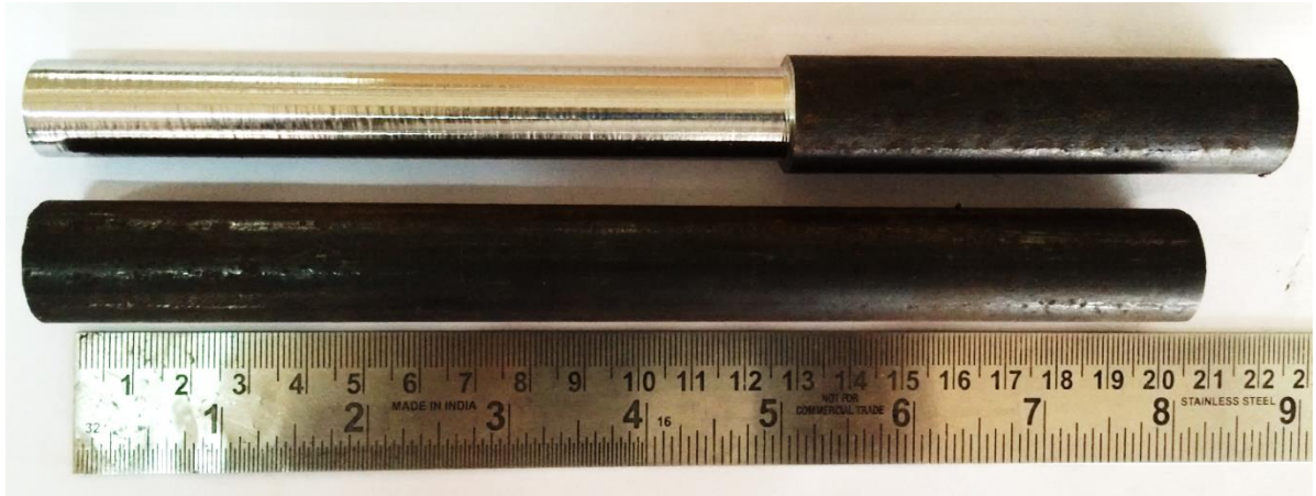
Fig.4.5 Mild steel rod and turning has been done up to 12.5 cm
