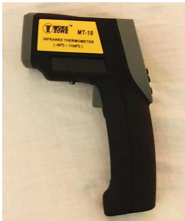
Fig.4.2 Non-Contact thermometer of Work Zome
