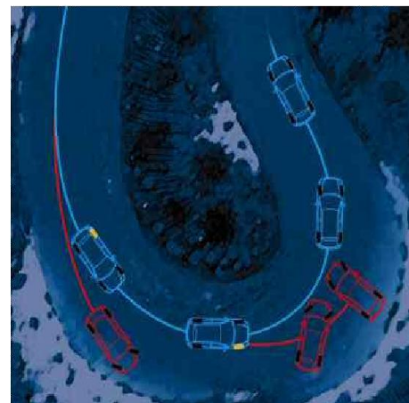
Figure 2.1: Ford's ESC. Stability-control systems utilize several sensors and a computer to determine the driver-intended path for a vehicle. The system will attempt to prevent a skid by applying individual wheel brakes.
