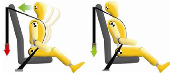
Figure 3.9: TRW's Active Control Retractor (ACR) unit takes the slack off the seatbelt moving the passenger into a safer crash position (left pic). During the collision or rollover, the ACR unit remains activated, keeping the passenger in a safe position (right pic).
