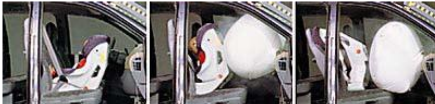
Figure 3.7: Rear-facing child restraints movement during airbag opening.
