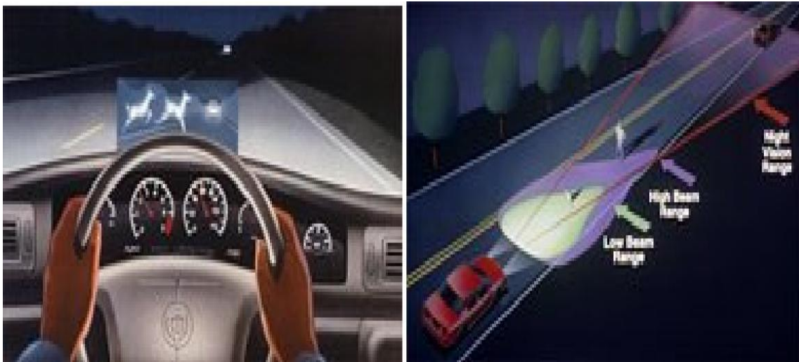
Figure 2.7: Night Vision allows the driver to see well beyond the reach of the car's headlights. This technology helps drivers detect and avoid potentially dangerous situations.
