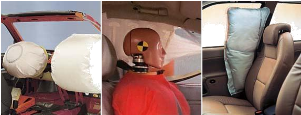
Fig.3.4 (a)Frontal dual airbag system (b)Side airbags to protect the head or head and torso
